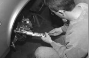
With a standard coil spring and shock configuration, Competition Engineering's 3-way adjustable drag shocks get the job done. Non back-halved cars have worked best with Smith Racecraft High-Energy springs and CE's drag shocks.
