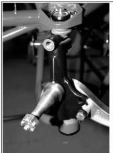
Chromemoly drop spindles for 67-69 Camaros and 68-74 Novas lower the cars height 2" for a low stance that makes a car look fast, even when it's sitting still. Lightweight standard spindles for 70-81 Camaros will be available soon.
