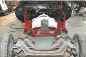
Smith Racecraft's tubular front subframes are accepted for competition by several racing organizations. The Nova pictured has seen improved 60 ft. times and lowered ET's due to the weight loss and improved front suspension, which gets the weight over the rear end quicker.
